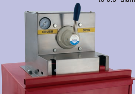
The Control Box, at top of unit.
