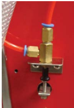
DOOR SAFETY SWITCH LOCATED ON BACK OF UFC550C and UFC850C
