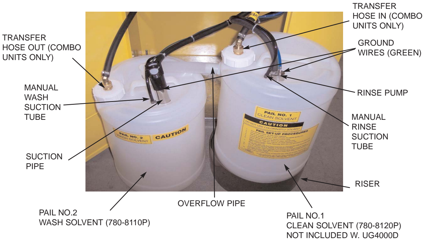
SOLVENT PAIL SETUP - PLASTIC PAILS
